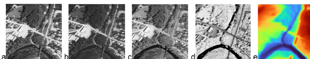
Figure 2. NAIP Imagery: a.Red, b.Blue, c.Green, d.Near-Infrared and e.DEM
